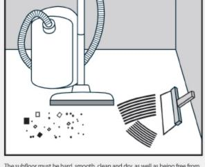
The subfloor must be hard, smooth, clean and dry, as well as being free from defects and fit for purpose. When required, scrape off and remove old adhesives and loose lay-ing leveling compound. Make sure the subfloor is flat and free from chemical substances and other contamination.
