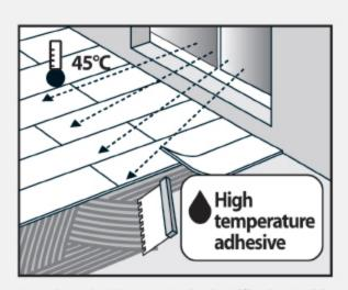
In areas that may be subject to excessive direct heat 45  $^\circ$ C or above (e.g. fully glazed sun facing conservatories) the floor must be installed with high temperature adhesive.
