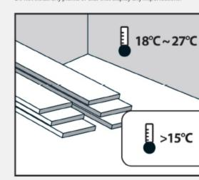
Product should be installed with a room temperature of between 18  $^{\rm T\!C}$  and 27  $^{\rm T\!C}$  and a floor temperature of above 15  $^{\rm T\!C}$  .
